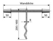
Spacer as formwork stop.
