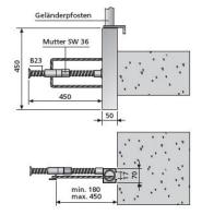
Guardrail post holder for accommodating BETOMAX® guardrail posts on the superstructure edges of bridges.
