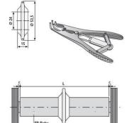
Swellable SD type water stop to prevent the ingress of water. Fitted using BETOMAX® SD installation pliers.
