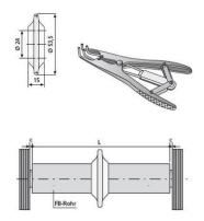
Swellable SD type water stop to prevent the ingress of water. Fitted using BETOMAX® SD installation pliers.
