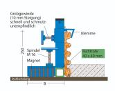
The MK 3 magnetic clamp is used to attach formwork profiles to steel formwork. They are used for shuttering balcony upstands, wall and ceiling end formwork as well as door and window recesses. The standpipe is firmly welded. Profiles up to a width of 250 mm can be clamped in the magnetic clamp. The uprights can also be supplied in a higher version on request.
